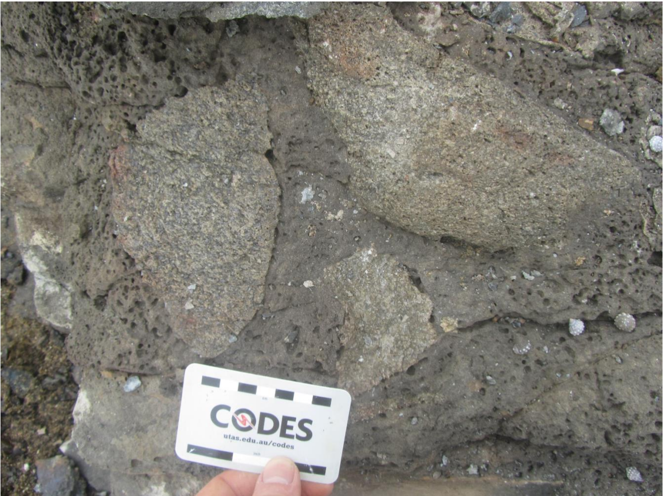
Gabbroic xenoliths in dyke SA-17-18
